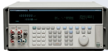
▲ AC reference standard (e.g. FLUKE 5720A)
